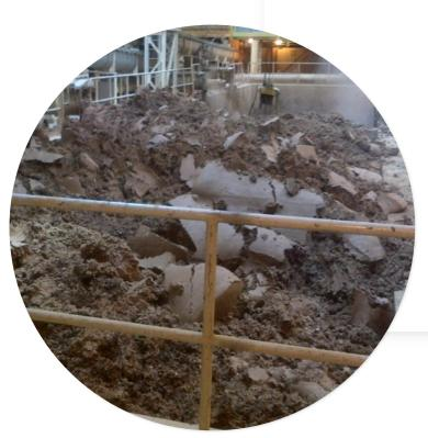
Biosolids without thermal hydrolysis treatment
